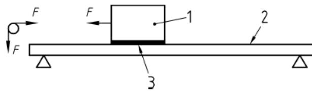
Figure 3: Test to establish coefficient of friction
