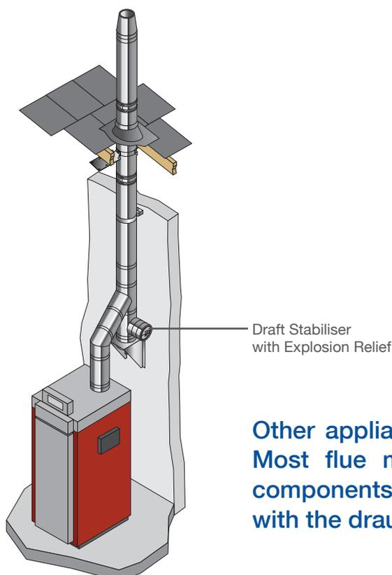
Other appliances make use of third party components. Most flue manufacturers can supply explosion relief components. The explosion relief is usually combined with the draught stabiliser.
