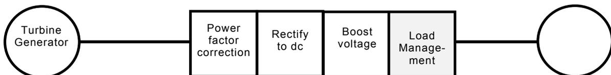
7.1.2 Inverter with passive rectifier and voltage boost
