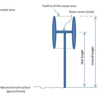
Typical horizontal axis wind turbine (HAWT)
